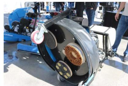
With a very innovative take on grinders, Prep Tech Systems has come up with an interchangeable grinding system that should entice small business owners trying to build up their fleet. The company has 25-, 30- and 34-inch heads that all fit on the same-size frame. So rather than buying a complete machine if you need something larger or smaller, you can simply purchase the needed head.
