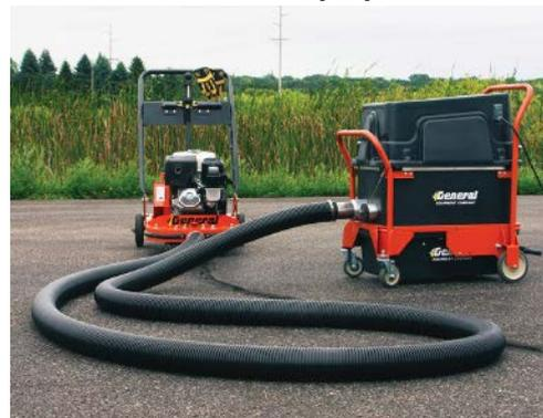
Featuring a 99 percent efficient at 0.5 micron prefilter and a 99.7 percent efficient at 0.3 micro HEPA secondary filter, the VS220 captures fine dust particles, allowing users to comply with OSHA respirable crystalline silica exposure regulations (OSHA 29 CFR 1910.1153). The unit includes separate 2- and 3-inch diameter dust-port connections for either simultaneous or independent operation.
