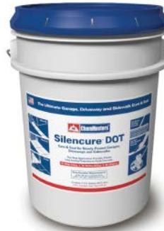
The compound cures concrete to ASTM C309 standards. Its white pigmentation provides a minimum 65 percent light reflectance to keep concrete cool as it cures, while integral silane meets most state DOT requirements for reduction of water and chloride ion penetration per NCHRP Report Series II & Series IV.
