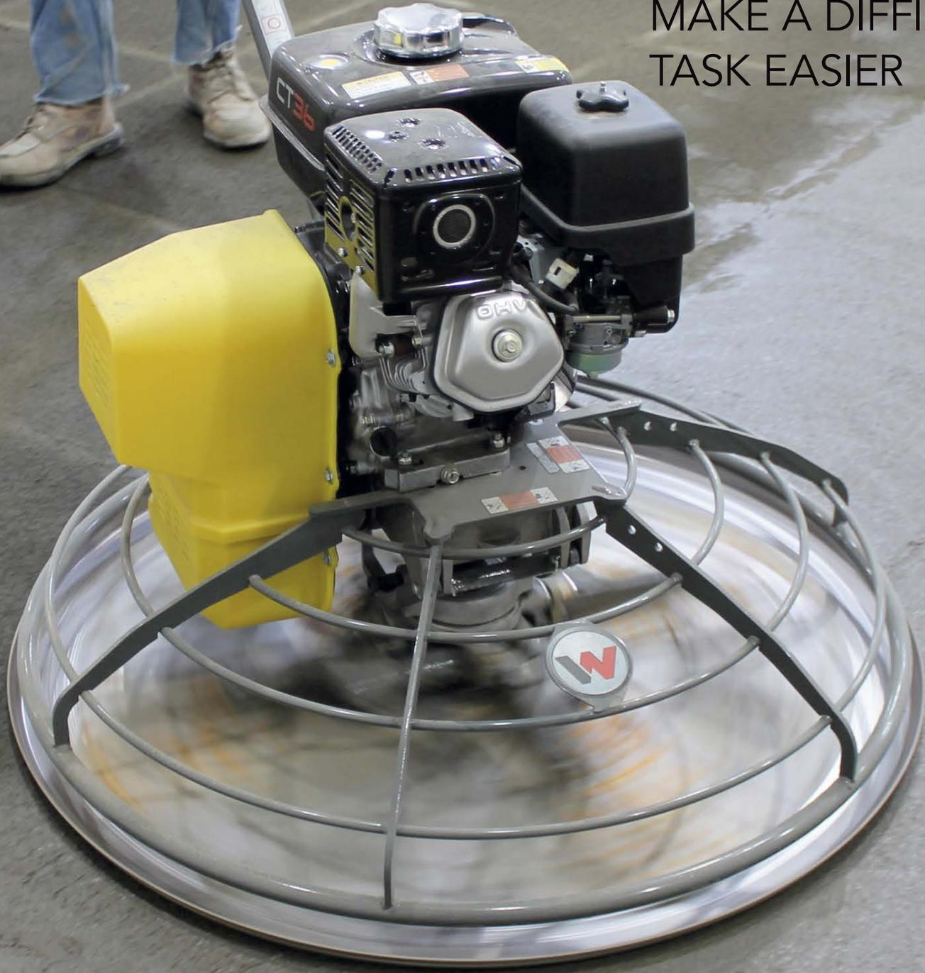
A power trowel can save time and manpower on jobs as small as 1,000 square feet. Its main advantage, though, is not letting the pour get ahead of you.
