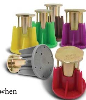
**Deck Insert** — Metal deck forms are corrugated and the placement of the anchors must be exact according to the design of the project. The new DDI insert solves this common issue and allows a cast-in-place insert to be placed on any surface of the deck including the incline where traditional metal deck inserts cannot be installed.
