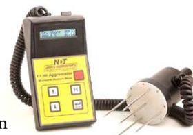
The prongs of the probe are inserted into the material to be tested and the percentage of moisture content is instantaneously shown on the easy-to-read display. On average, five to 10 readings are normally taken to ensure a valid result. This output is converted by the integrated microprocessor and the moisture content is displayed directly as a percentage of dry weight.
