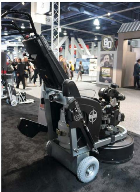
**HTC** ([www.htc-floorsystems.com](http://www.htc-floorsystems.com)) launched its first propane grinder at the show, the 800 RXP. Except for its power source, it's almost identical to the popular remote-controlled 800 RX electric model but goes one better. Designed with ergonomics in mind, the new four-head 800 RXP offers up to 50 percent higher productivity. A floating grinding cover helps reduce airborne dust. Expect more propane products to follow, a spokesman says.
