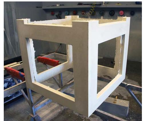
The inside of the table wasn't finished to the same degree as the outside. While the outside didn't have exposed fibers, the inside did. This didn't matter since the inside wasn't going to be very visible. For the inside, I used a pneumatic diamond polisher with a 50-grit pad, then 100 and finally 200.
