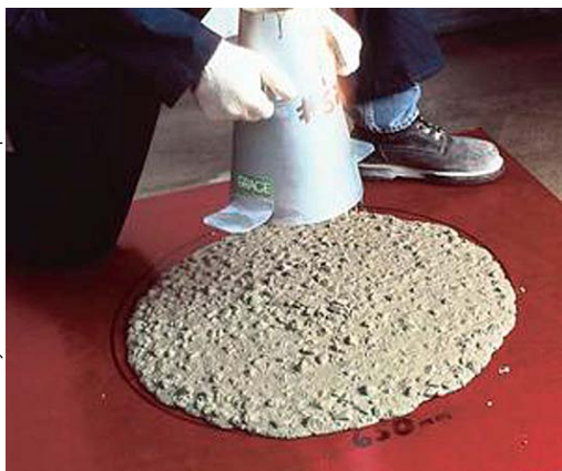
A slump flow test showing the spreading characteristics of self-consolidating concrete.
