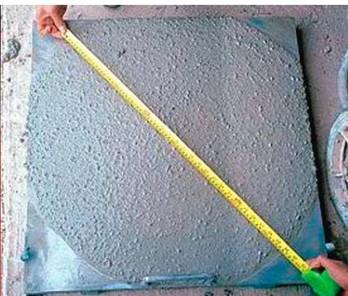
A slump flow test showing the spreading characteristics of self-consolidating concrete.
