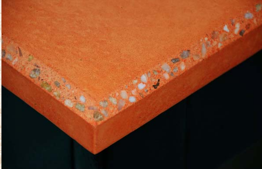
A bevel-profiling wheel was used to cut the angle in this edge and expose the aggregate.
