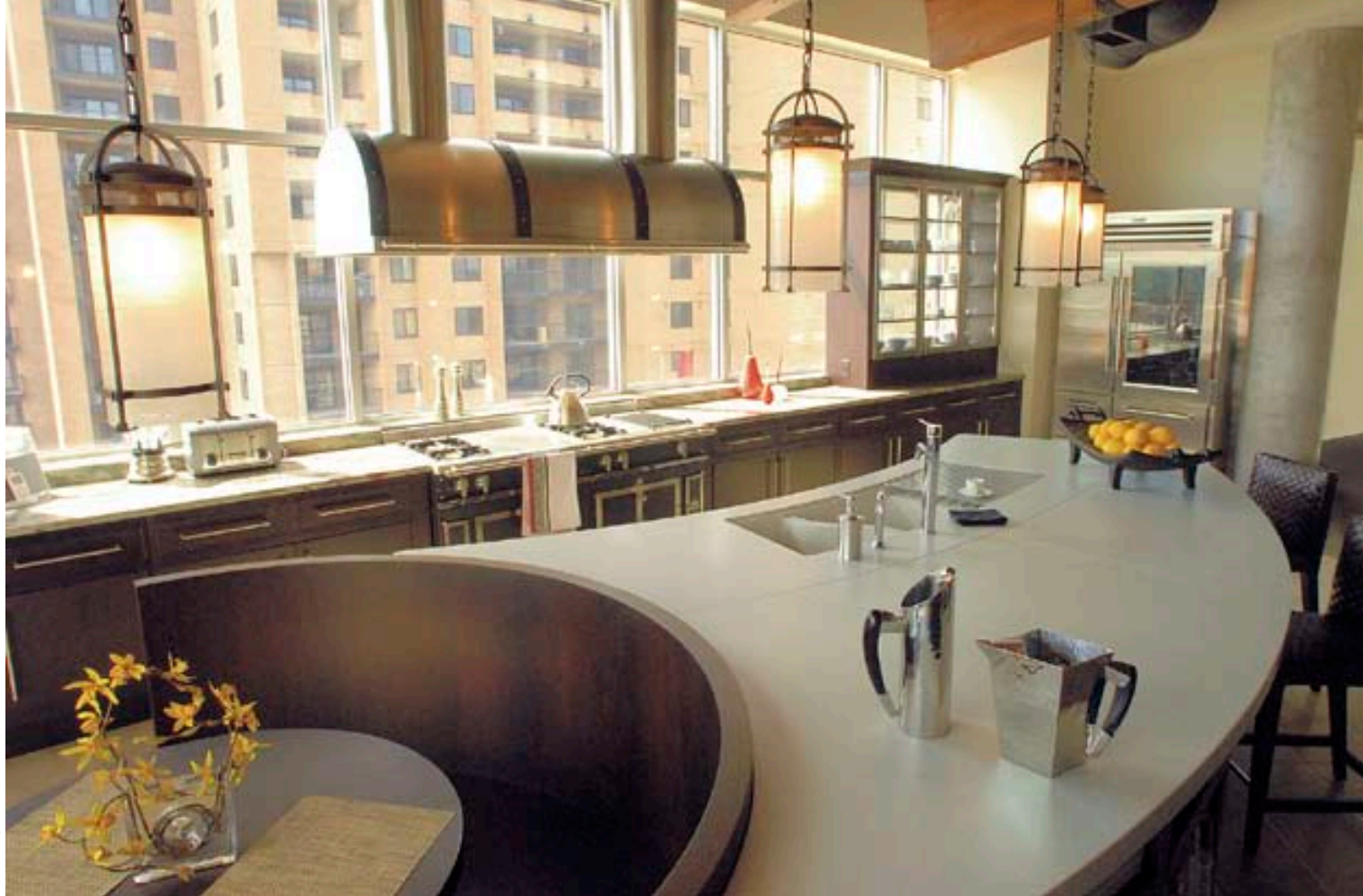
The EarthCrete family of concrete mixes incorporates recycled paper fibers, ceramics and industrial by-products.
